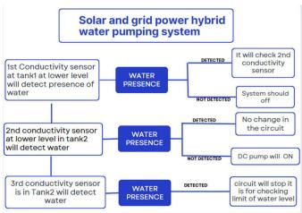
Tank 1 comprises the first conductivity sensor installed at the lower level of the tank. It detects the water level in the tank. When the water level is measured, the system proceeds to check the second conductivity sensor. Within a relation, if no water is measured, the system will be turned off to save power.
