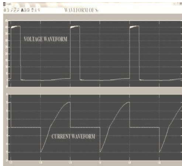
Figure 7: Output waveform of switch S 2
